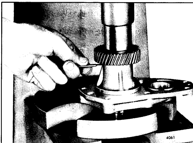
Fig. 17 - Installing Blower Drive Gear on Shaft
