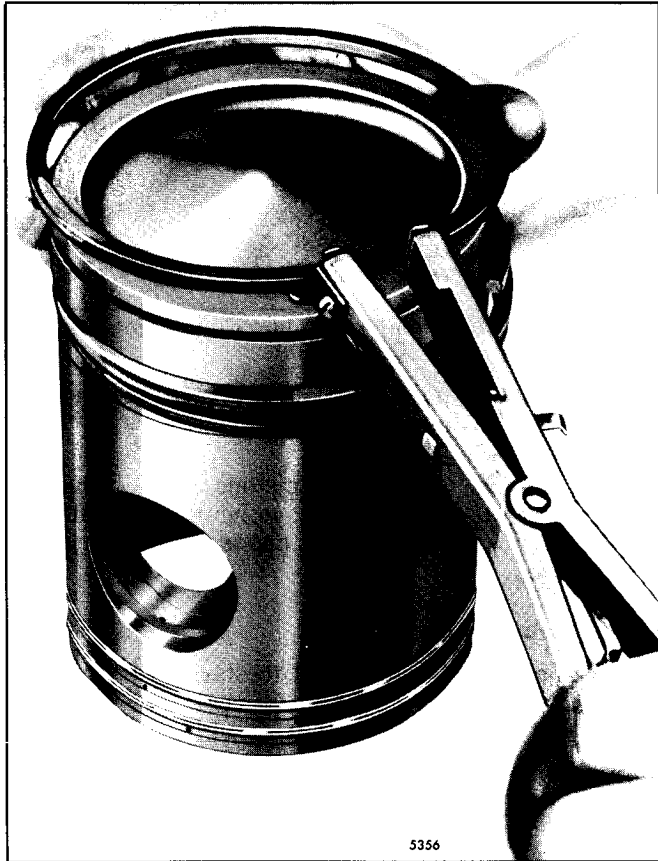
Fig. 13 - Removing or Installing Piston Rings with Tool J 8128
