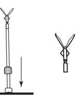
4. Pull the insert out of the shaft. Now you will have 3 separate pieces: a handle, a shaft with a nut, and an insert.
