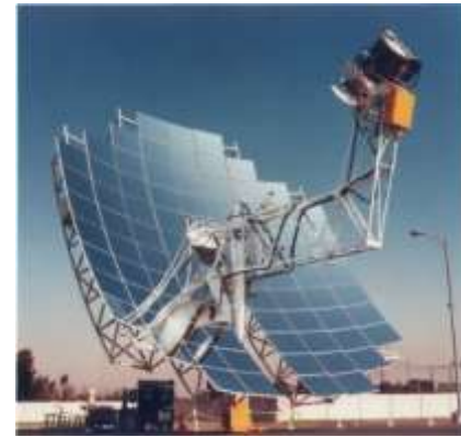
Figure 2: Stirling engine in conjunction with solar concentrator
