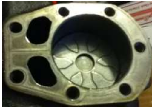
Figure 11: View under the caps of the compressor
