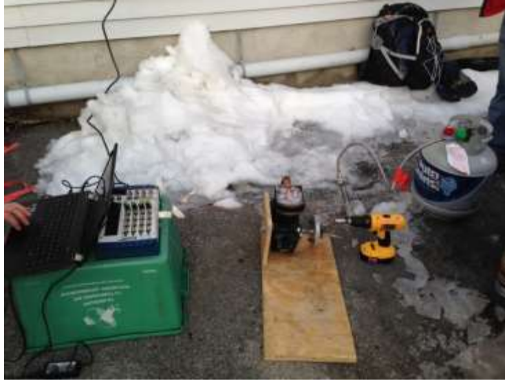
Figure 32: Testing the engine with the propane burner, drill, and DAQ box
