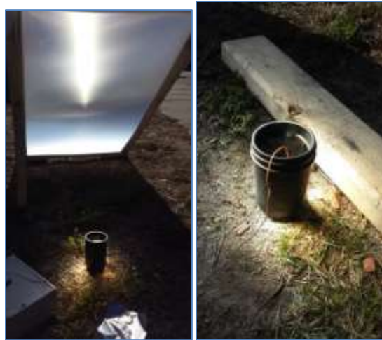
Figure 25: Heat Measurements Taken with Thermocouple
