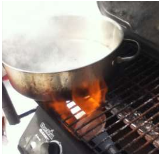
Figure 27: Testing the propane burner by heating a pan of water to boiling
