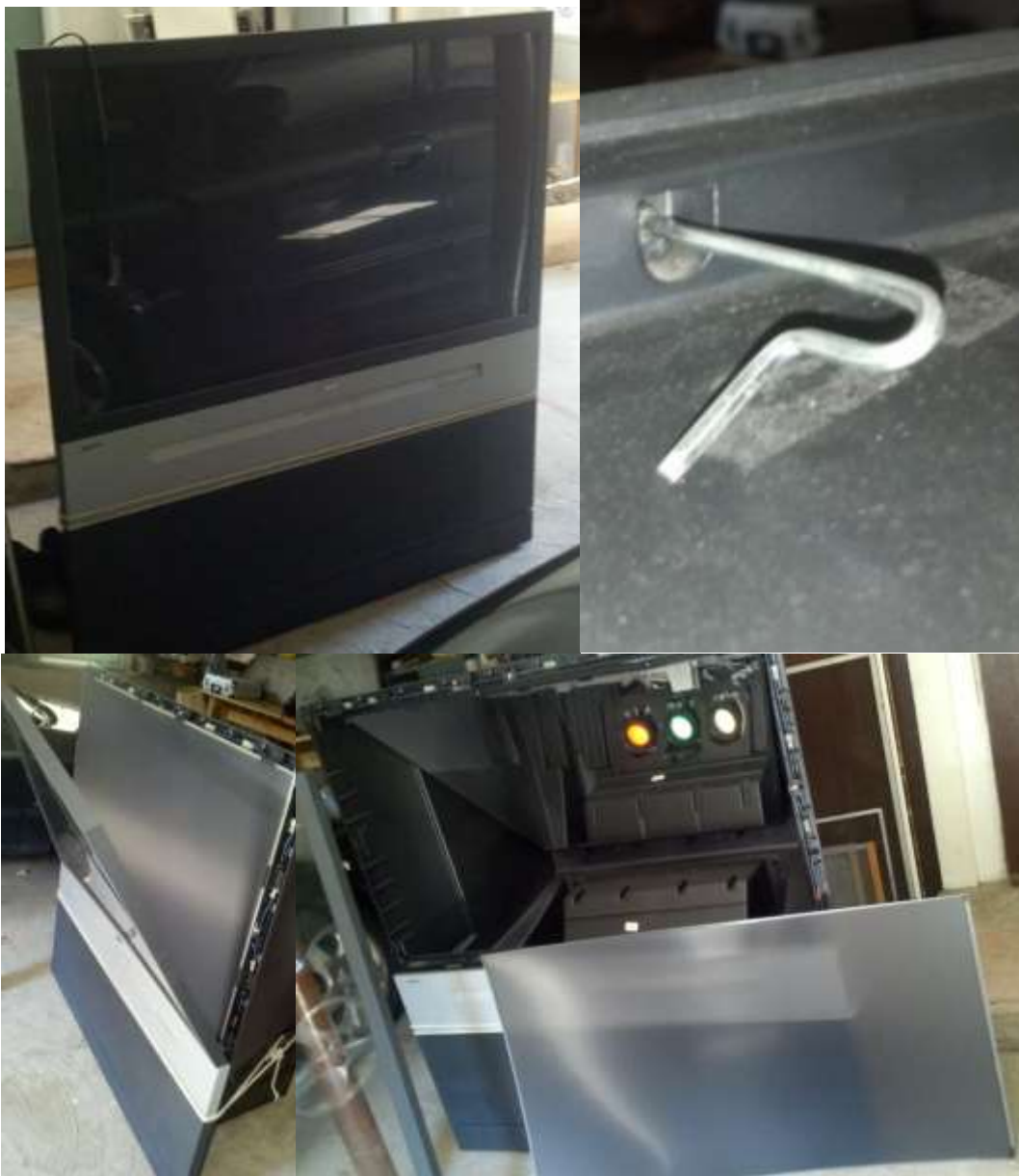
Figure 21: Rear Projection TV (top left), Removing Outer Frame (Top Right), Outer Frame Coming Off (Bottom Left), and Fresnel lens Removed (Bottom Right).
