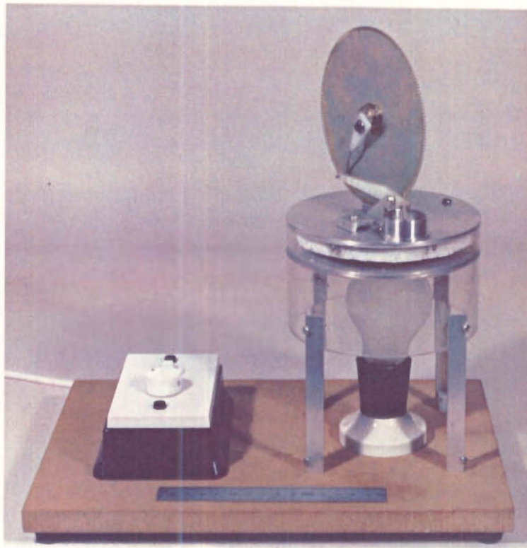
Photo 6.1 (a) DMC with heat exchangers fitted and dynamometer fitted. (b) Low delta T engine used for demonstrations.
