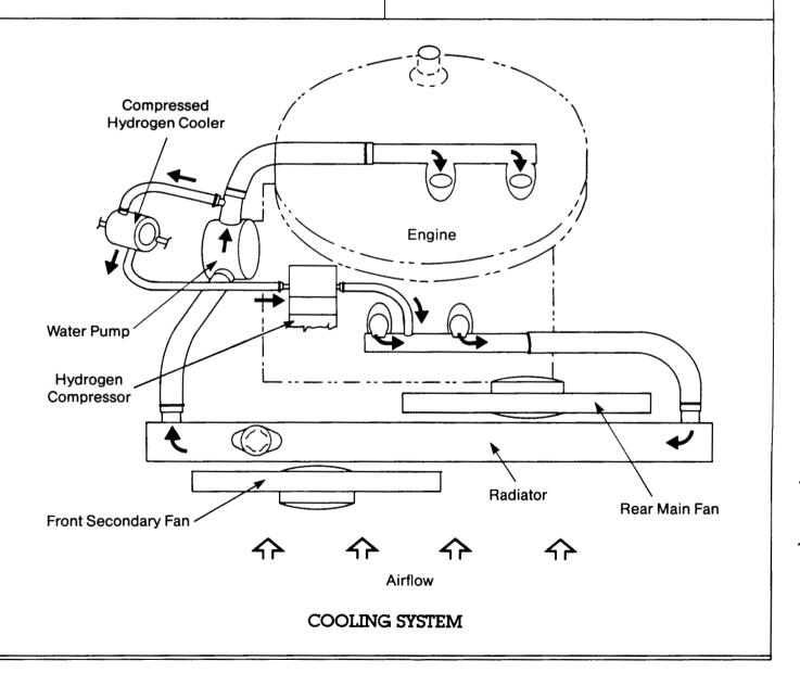
small parallel pass, connected by standard small-diameter heater-supply hose. The entire loop is intentionally kept nonpressurized by a vented overflow tank and nonspring radiator cap in order to preclude the cavitation that might otherwise occur from the suction of the positive-displacement pump.
