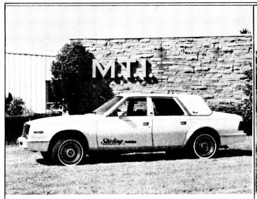
Stirling-Powered AMC Concord Demonstration Vehicle
