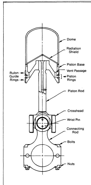
The wrist pin is machined from low-alloy steel. A radial hole is bored through the center to accommodate the shank of the piston rod as it is threaded into the crosshead. The wrist pin acts as the journal in the upper end bearing of the connecting rod and has a hardened, polished surface. This bearing is lubricated with excess oil initially sprayed at the piston rod to lubricate and cool the pumping Leningrader seal.
