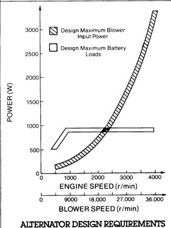
The blower motor control converts the alternator output to a variable dc level by a three-phase bridge rectifier and feeds it to the blower motor. For upstart, the battery simply replaces the dc voltage supplied by the alternator.
