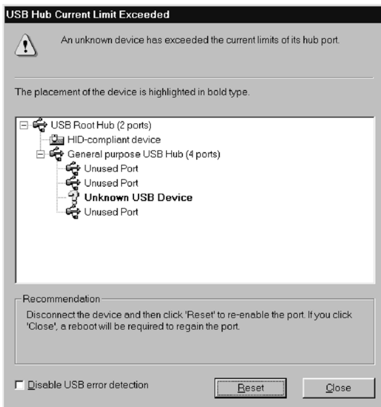
Figure 16-3. When a device exceeds the current limit of its hub's port, Windows warns the user and offers assistance.
