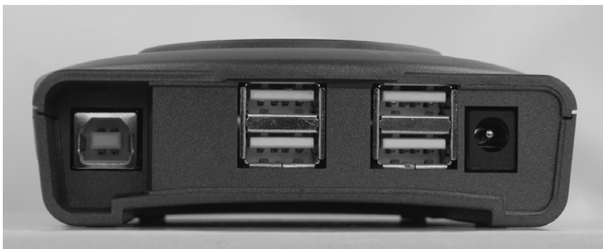
Figure 15-1. This hub has an upstream-facing port with a Standard-B receptacle (left), four downstream-facing ports with Standard-A receptacles (center), and a power connection (right).
