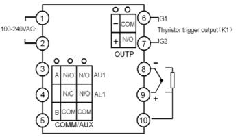
used for AU1 or AU2 alarm output; if set parameter bAud = 2, it can be used for AU1 or AL1 alarm output. If L1, L2, L4, G, K1, W1 or W2 is installed, it can be the auxiliary output in bidirectional (heating/refrigerating) control (Auxiliary output doesn't support analog current output); if I2 is installed and bAud = 1, then it can input on-off signal to switch SP1 and SP2 (AI-516) or switching the program status RUN / Stop (AI-516P) by connecting a switch between terminals number 3 and 5.
