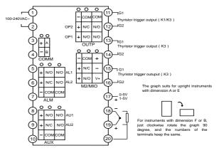
Note 4: When main output selected linear current or SSR voltage, output form terminal 13+, 11-,
