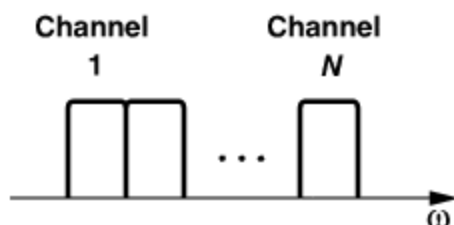
Figure 3.51 Frequency-division multiple access.
