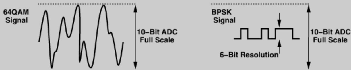
Figure 13.3 Available ADC resolution for a full-scale signal and a smaller input swing.
