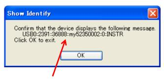
You'll see the VISA address of the unit on the software and the instrument GUI
